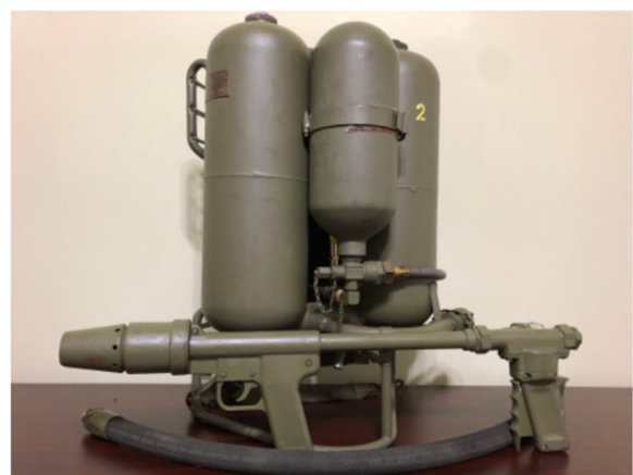
Fig. 2 The M2–2 man-portable flamethrower utilized by the U.S. military in the Pacific theater during the last 2 years of WWII. The example is working unit from the author’s personal collection. The original hex shaped gas caps, rupture disks and vent tube have been replaced with the more reliable and safe vented fuel caps developed in 1953
